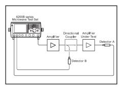
Test Set up for Ratioed Measurements
