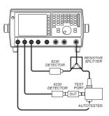
Filter measurement with live reference
